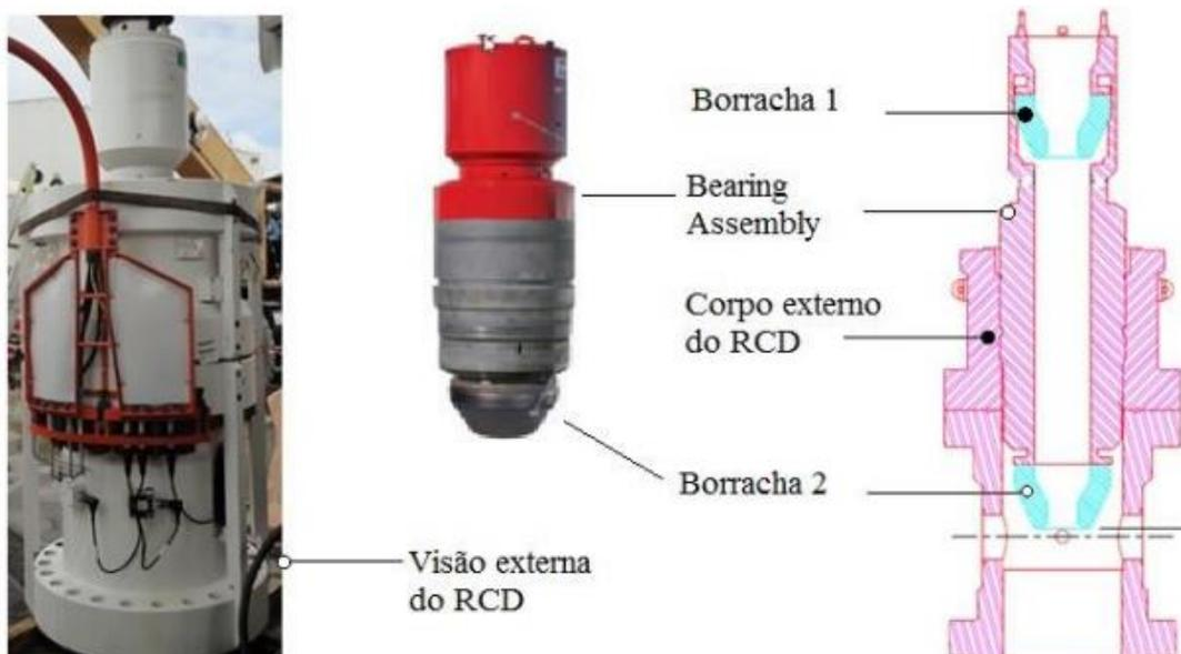
Figura 105: Bearing Assembly
