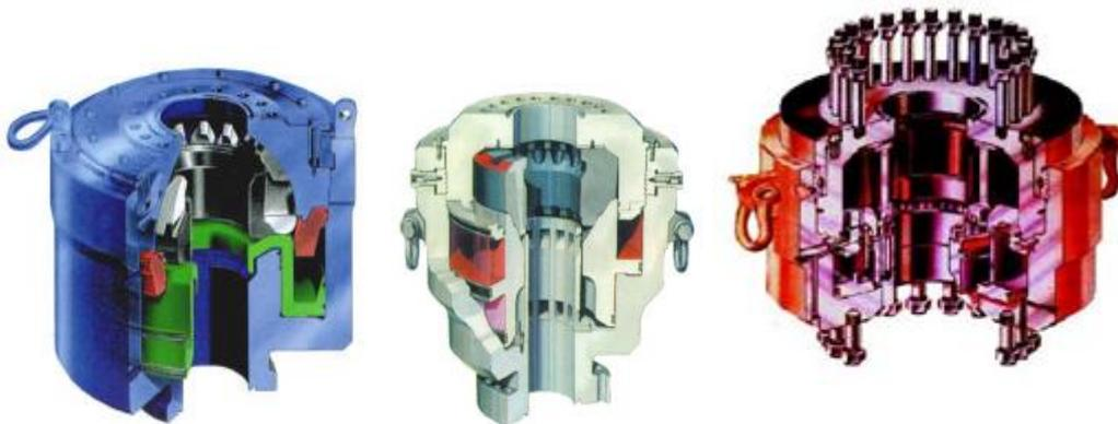
**Figura 6 - (a) Anular Shaffer (b) Anular Hydril (c) Anular Cameron Tipo D**
