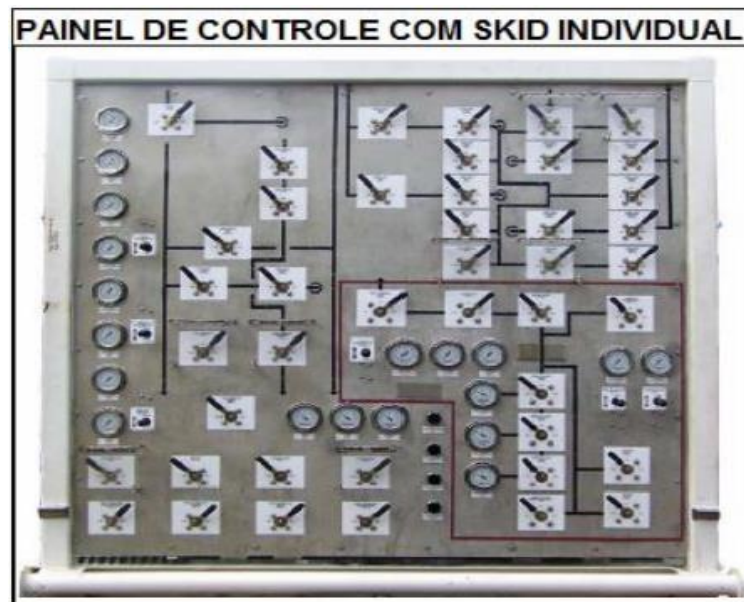
Figura 16: Painel de controle com skid individual
